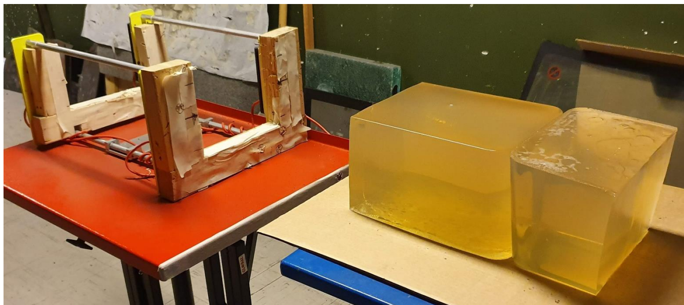
Test 2: Setup to measure the velocity after penetrating 450mm gelatin.
