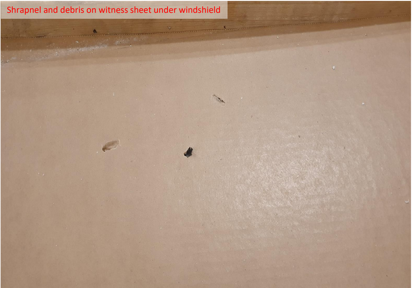
Shrapnel and debris on witness sheet under windshield
